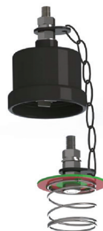
Failed- arrester disconnected
