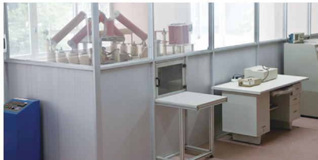
Multi-onda Generator Surge
