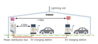
SCENE 3 SPD for outdoor EVSE – with lightning protection system (LPS)
