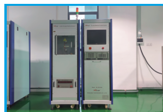
AC/DC Thermal Stabilizer System Thermal Stabilizer Control System
