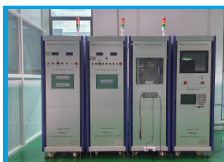
Combination Wave Generator GCW Measurement Control System AC/DC Operating Duty Power Supply 100A AC Operating Duty Power Supply
